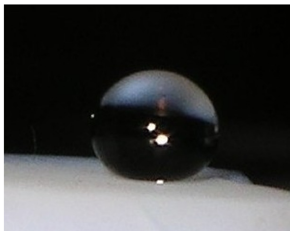
Fig. 7. The photograph showing an increase in the sphericity of the water droplet from MTMS to TMMS treated aerogels.
